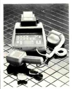
THE MEDTRONIC PACEMAKER programmer and two of the small Spectrax-SX pacemakers
