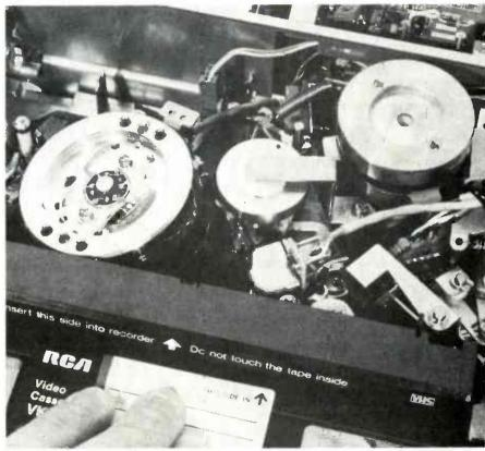
WITH SIDE, TOP AND BACK COVERS OFF cassette carrier—chamber that holds cassette—becomes accessible. Removing four screws frees carrier cover. Pawl trips latch at end of cassette gate, a door in the cassette itself that protects tape inside, and, as carrier is pressed down, metal post near corner lifts gate to uncover tape at front of cassette.
