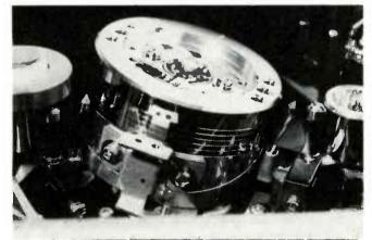
**TAPE POSITIONING** in transport can be critical. Guides and posts along path take care of that positioning. However, probably the most crucial are guide posts on loading rings (photo above). They align tape with respect to head wheel and thus with spinning video heads. Even slight misadjustment of just one guide post delivers band of snow (photo above, right). In some cases, you see multiple bands across picture. This symptom may not be too bad with tapes recorded on same machine.
